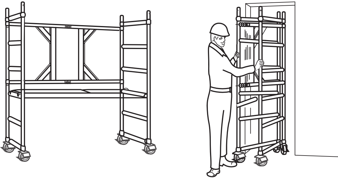
Figure 4 — Example of a room scaffold
